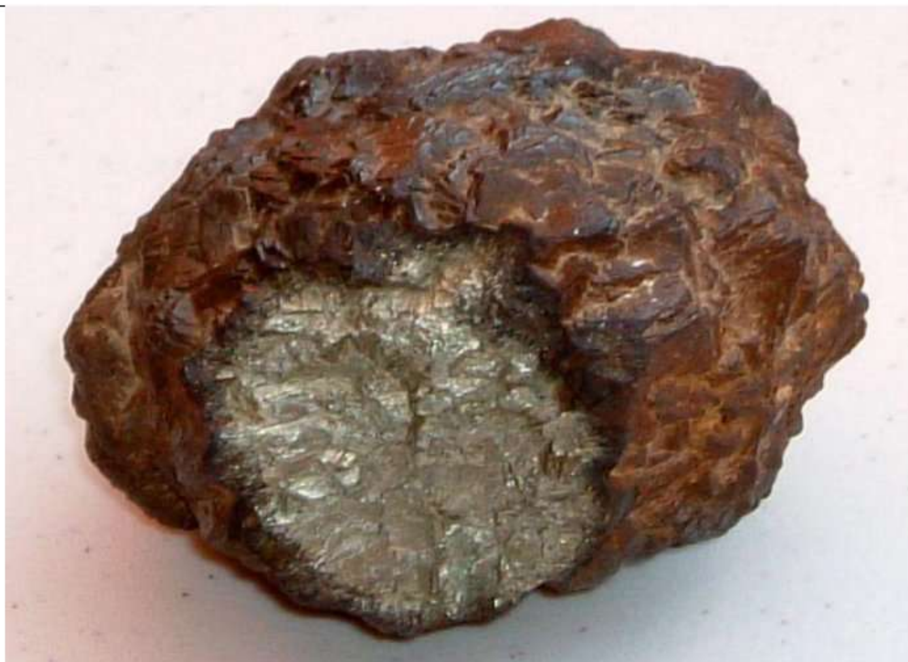
Cluster of pyrite crystals. The outside is rusty because the iron sulfide has oxidized to iron oxide.
