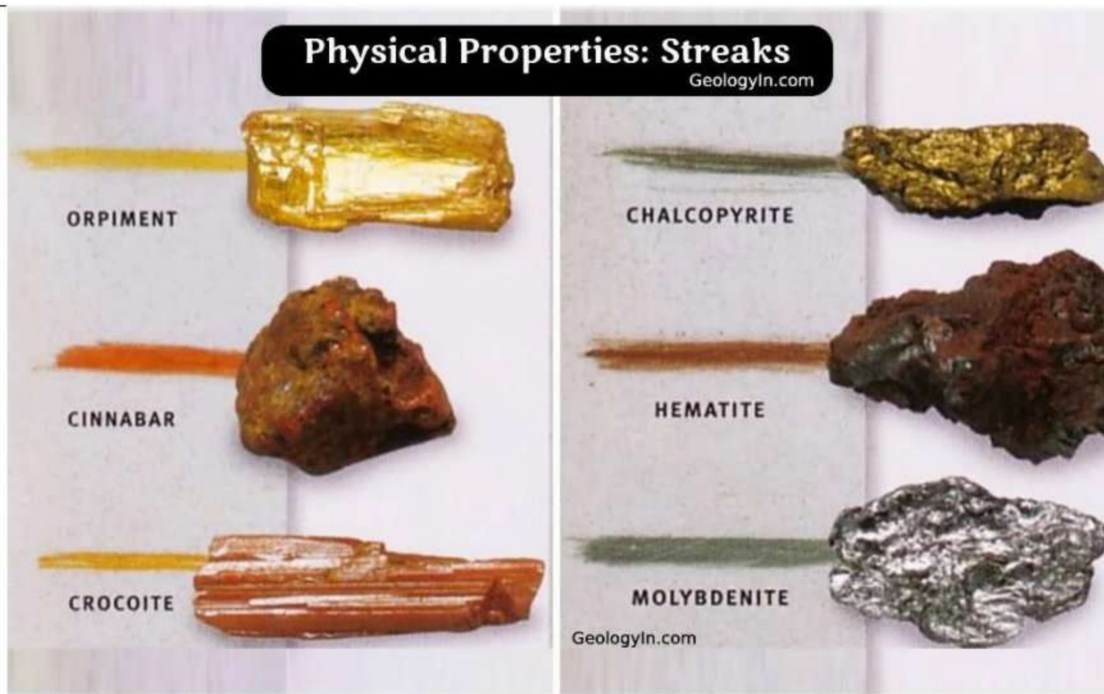
Mineral streak tests showing the colour of the mineral powder
